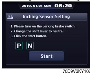
Before starting calibration, press the START button when the parking switch is turned on and the gear is in the neutral state.
